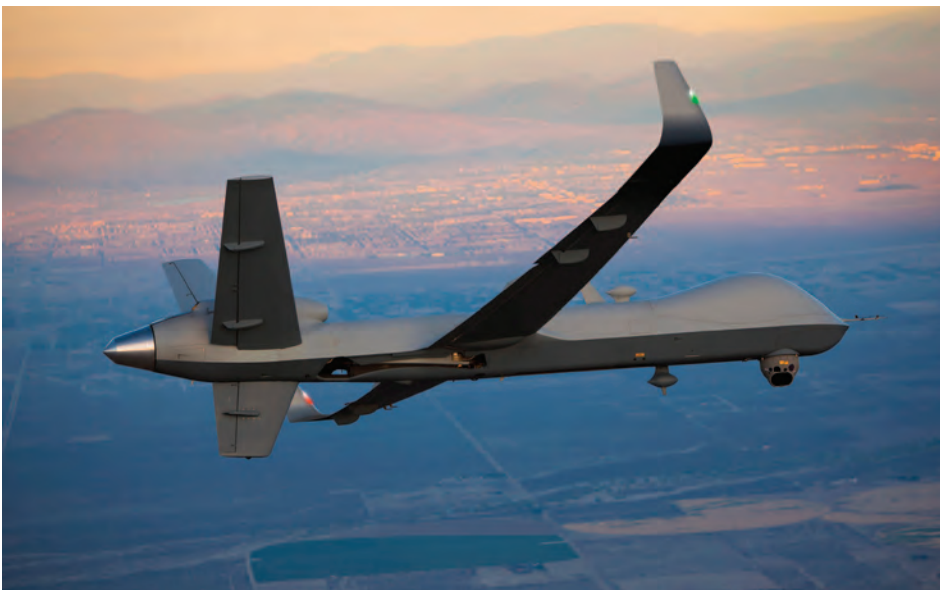
Predator B testbed flying with the long-span wings that provide Certifiable Predator B with over 40 hours of flight endurance
