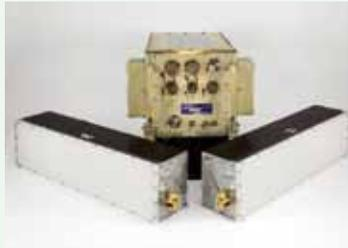
The GA-ASI-developed Detect and Avoid (DAA) system is made up of an Air-to-Air Radar, TCAS II, ADS-B IN/OUT, and a Conflict Prediction and Display System. The DAA system provides pilots with real time situational awareness about proximate traffic and real time guidance to 'remain well clear'.
