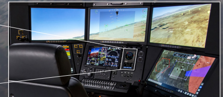
GA-ASI's Certifiable Ground Control Station (CGCS)
