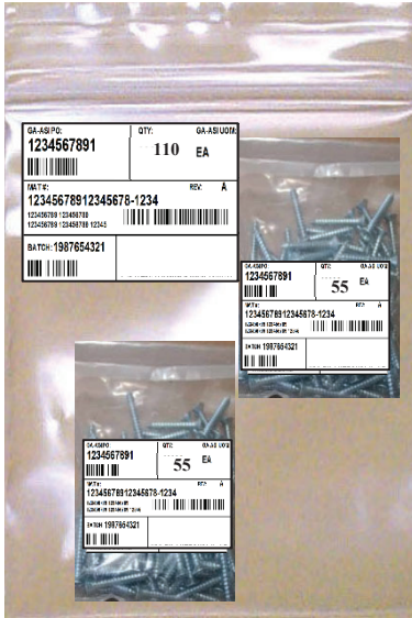
Figure D-4 Single Line Item in Separate Packages within another Package. (Option 1: Single label on outer package with full/total quantity amount).
