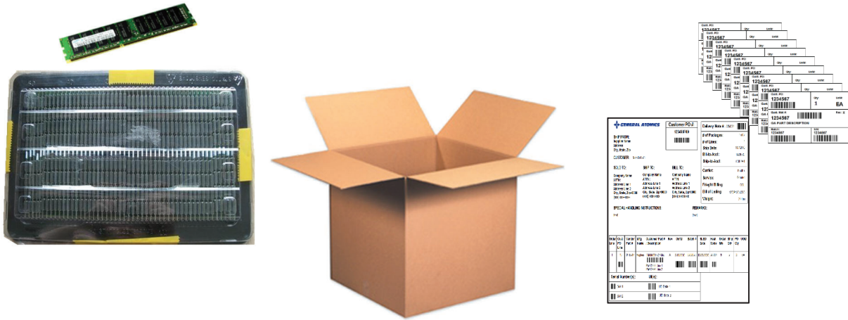
Figure D-8 Multiple Serialized Parts within same Package (Unpeeled label(s) attached to packing slip).
